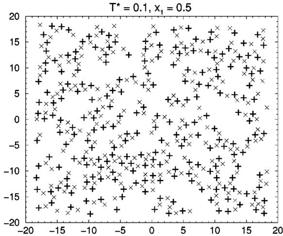
FIG. 21. The final configuration of the equimolar binary mixture ( $\sigma_2/\sigma_1=1.4$ ) at  $T^*=0.1$ , showing only the positions of the particles which are not six-coordinated as determined by the Voronoi analysis described in Sec. V C. At this temperature, all of these defects consist of only five-coordinated small particles ( $\times$ ) and seven-coordinated large particles ( $+$ ).
