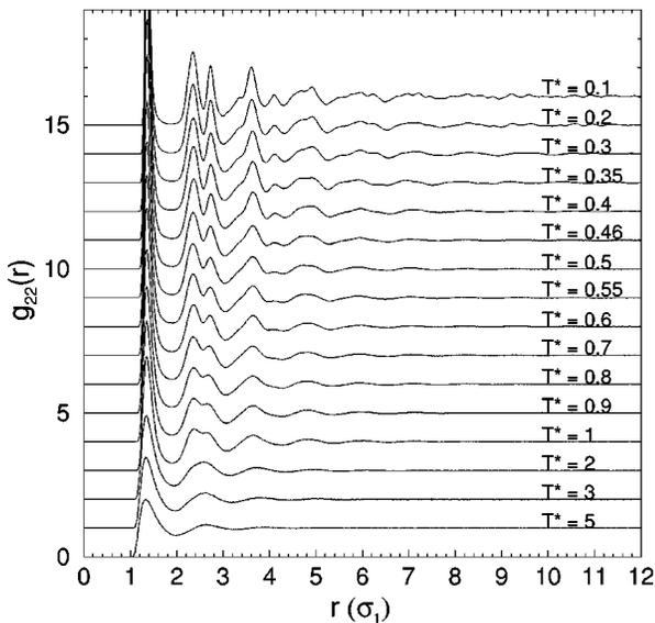
FIG. 5. The partial pair distribution function  $g_{22}(r)$  as a function of distance from  $T^*=5$  down to  $T^*=0.1$  for the equimolar binary mixture with  $\sigma_2/\sigma_1=1.4$ . For  $T^*\leq 3$ , each curve has been shifted upwards by one unit from the higher temperature curve directly preceding it.
