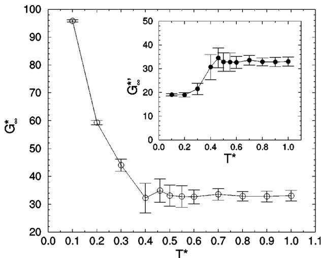
FIG. 26. The infinite frequency shear modulus  $G_\infty^*$ , calculated using Eq. (31), for the equimolar mixture over  $0.1 \leq T^* \leq 1.0$ . The insert shows the temperature dependence of the shear modulus minus the contribution from the mean shear stress as discussed in the text.
