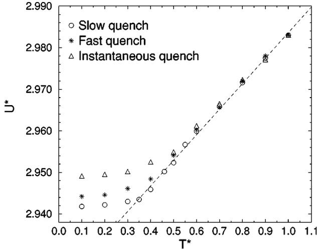
FIG. 19. The temperature dependence of the potential energy per particle  $U^*$  of the equimolar binary mixture ( $\sigma_2/\sigma_1=1.4$ ) for three different cooling rates as described in Sec. V B. The MD data for the slow quench is also listed in Table I. The dashed line is a linear regression through the results for the slow quench in the temperature range  $0.4 \leq T^* \leq 1$  where the system is able to reach equilibrium.
