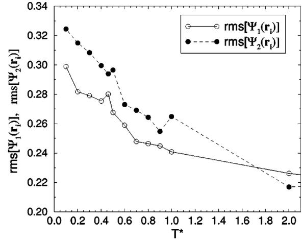
FIG. 12. The temperature dependence of the root mean square (rms) deviations of the local hexagonal order parameters  $\Psi_1(\mathbf{r}_j)$  and  $\Psi_2(\mathbf{r}_j)$  for the equimolar binary mixture.
