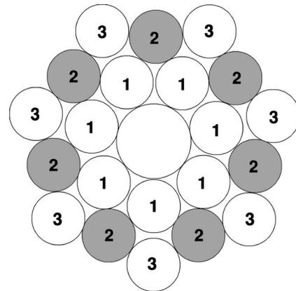
FIG. 27. Packing of hard discs about a large disc indicating the first, second, and third solvation shells as discussed in the Appendix.
