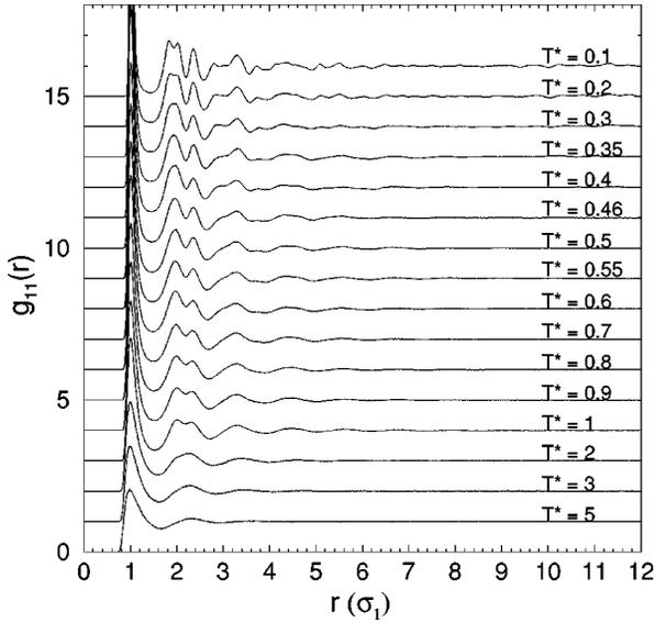
FIG. 4. The partial pair distribution function  $g_{11}(r)$  as a function of distance from  $T^*=5$  down to  $T^*=0.1$  for the equimolar binary mixture with  $\sigma_2/\sigma_1=1.4$ . The pair distribution functions have been constructed with a spatial resolution of  $0.01\sigma_1$ . For  $T^*\leq 3$ , each curve has been shifted upwards by one unit from the higher temperature curve directly preceding it.
