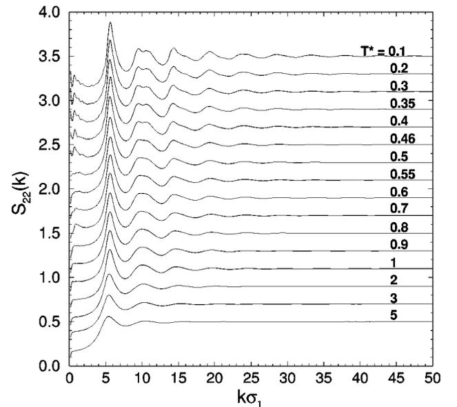
FIG. 9. Partial structure factor  $S_{22}(k)$  for all temperatures investigated for the equimolar binary mixture with  $\sigma_2/\sigma_1 = 1.4$ . For clarity, each curve below  $T^* = 5$  has been displaced vertically by 0.2 units above the higher temperature curve directly preceding it.
