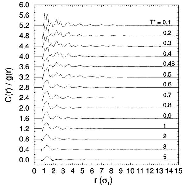
FIG. 13. The orientational correlation function  $C(r)/g(r)$ , as defined in the text, calculated for  $0.1 \leq T^* \leq 5.0$ . For very short distances less than interparticle separations, the function is undefined and has been set equal to zero. For clarity, functions have been offset vertically by 0.4 units above the preceding curve.
