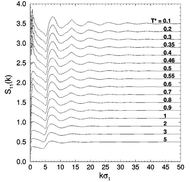
FIG. 8. Partial structure factor  $S_{11}(k)$  for all temperatures investigated for the equimolar binary mixture with  $\sigma_2/\sigma_1 = 1.4$ . For clarity, each curve below  $T^* = 5$  has been displaced vertically by 0.2 units above the higher temperature curve directly preceding it.
