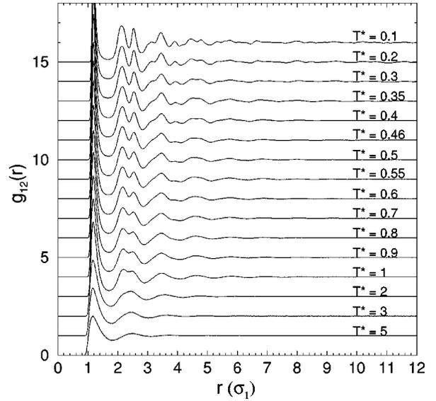
FIG. 6. The partial pair distribution function  $g_{12}(r)$  as a function of distance from  $T^*=5$  down to  $T^*=0.1$  for the equimolar binary mixture with  $\sigma_2/\sigma_1=1.4$ . For  $T^*\leq 3$ , each curve has been shifted upwards by one unit from the higher temperature curve directly preceding it.
