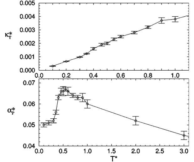
FIG. 23. The temperature dependences of the isothermal compressibility  $\kappa_T^*$  and the thermal expansion coefficient  $\alpha_p^*$  for the equimolar binary mixture with  $\sigma_2/\sigma_1 = 1.4$ .
