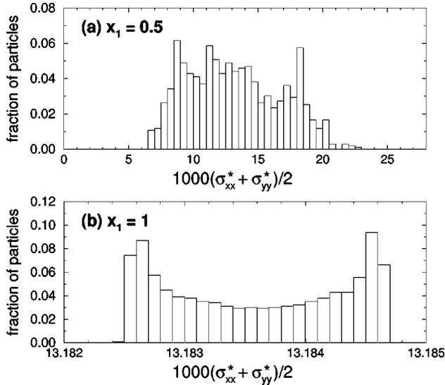
FIG. 25. The distribution of the local compression  $(\sigma_{xx}^* + \sigma_{yy}^*)/2$  for the amorphous binary mixture and the pure crystalline state at  $T^*=0$ . Again observe the difference in the horizontal scales.
